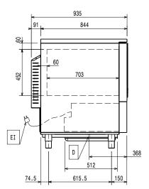
Drain Electrical inlet (power)
